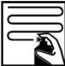
Apply 1 light/medium coat followed by a full coat to give 50 microns dry film thickness.
